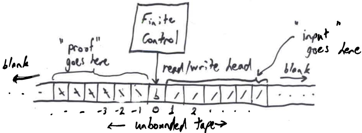
In one step, machine can write a symbol, move head one position, change state.
